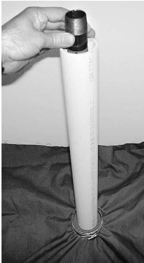
Figure 7 - Drop Tester just before making a test drop. Note that the guide tube is centered on the clamped fabric, and the drop probe is being used as a plumb bob to make the guide tube vertical.
