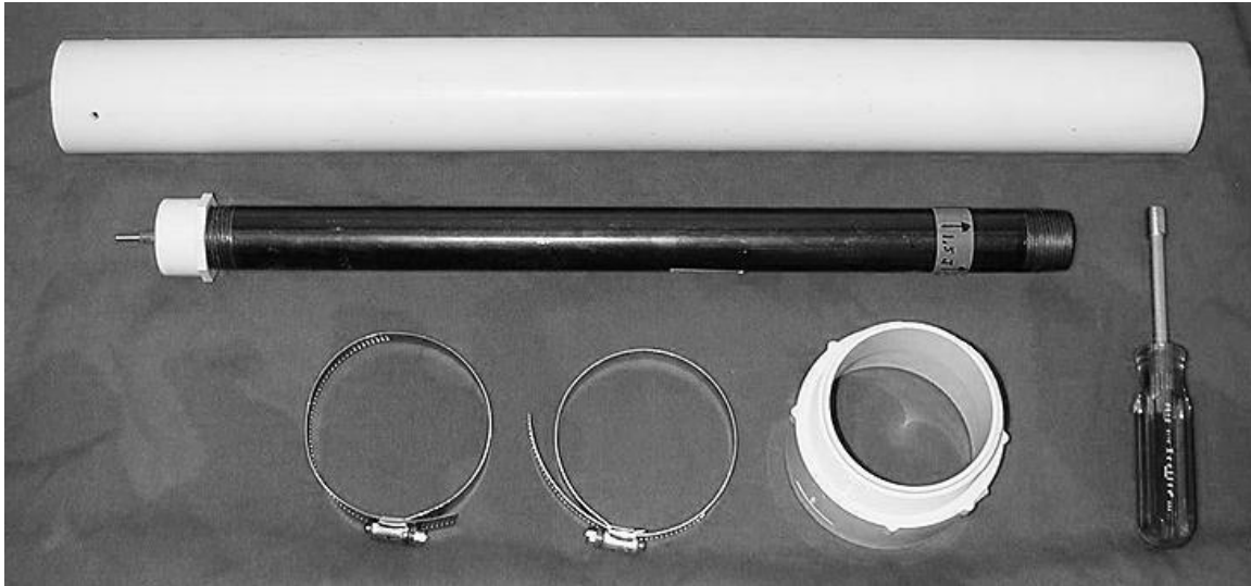
Figure 5 - Parts needed for SCA Standard Drop Tester for fencing armor.
