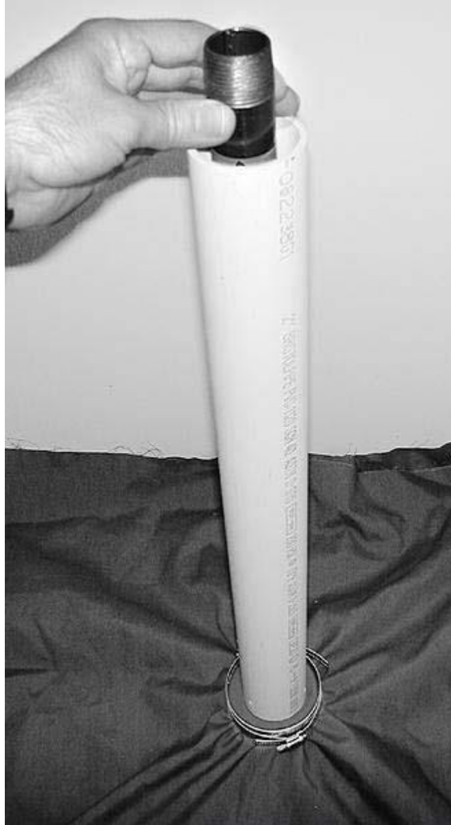
Figure 1 - Drop tester (pipe end sticking out of white guide tube) ready to use on some fabric clamped onto the 3" flange.
